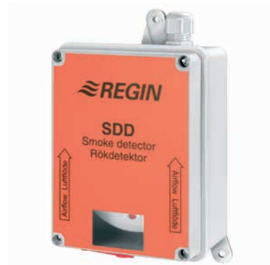
Figure 56: Smoke detector. Works on optical detection and has a built-in relay for alarming. When the smoke detector is activated, the unit stops as in case of fire.
