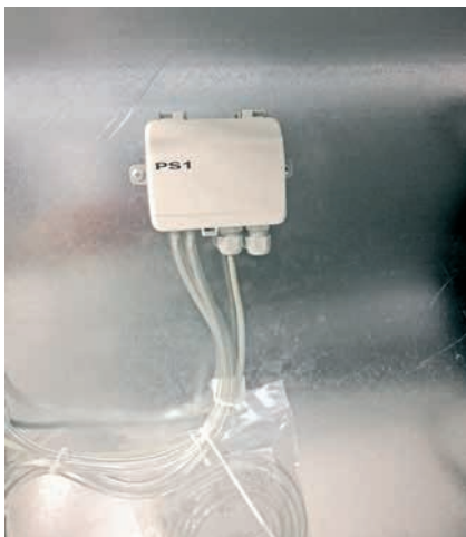
Figure 51: Pressure sensors unit with two differential pressure sensors. In CompAir it is used for measuring pressure in duct and also for measuring air flow of inlet and outlet fans. Communication with controller is via EXOline communication.
