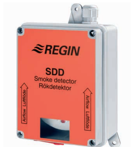
Figure 56: Smoke detector. Works on optical detection and has a built-in relay for alarming. When the smoke detector is activated, the unit stops as in case of fire.
