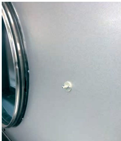
Figure 52: Tube connector for measuring duct pressure. User has to connect the attached tube to connector. The other end has to be connected to outlet air duct. The same procedure is required on inlet side. Inside CompAir, tubes must be connected to inside connectors.
